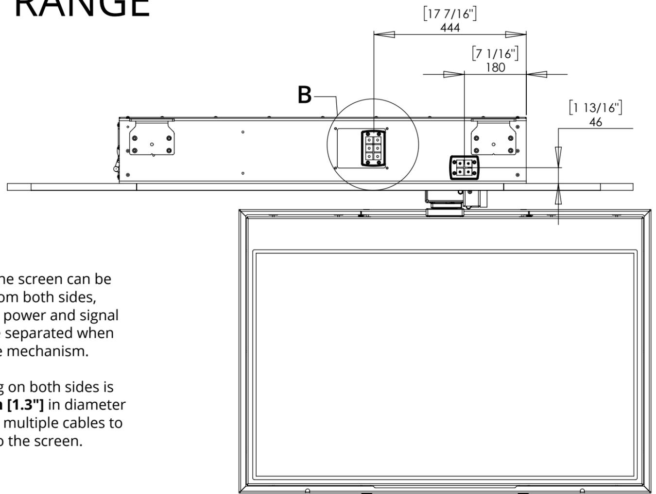
Cables pass through easily removable cable gland plates into mechanism.
