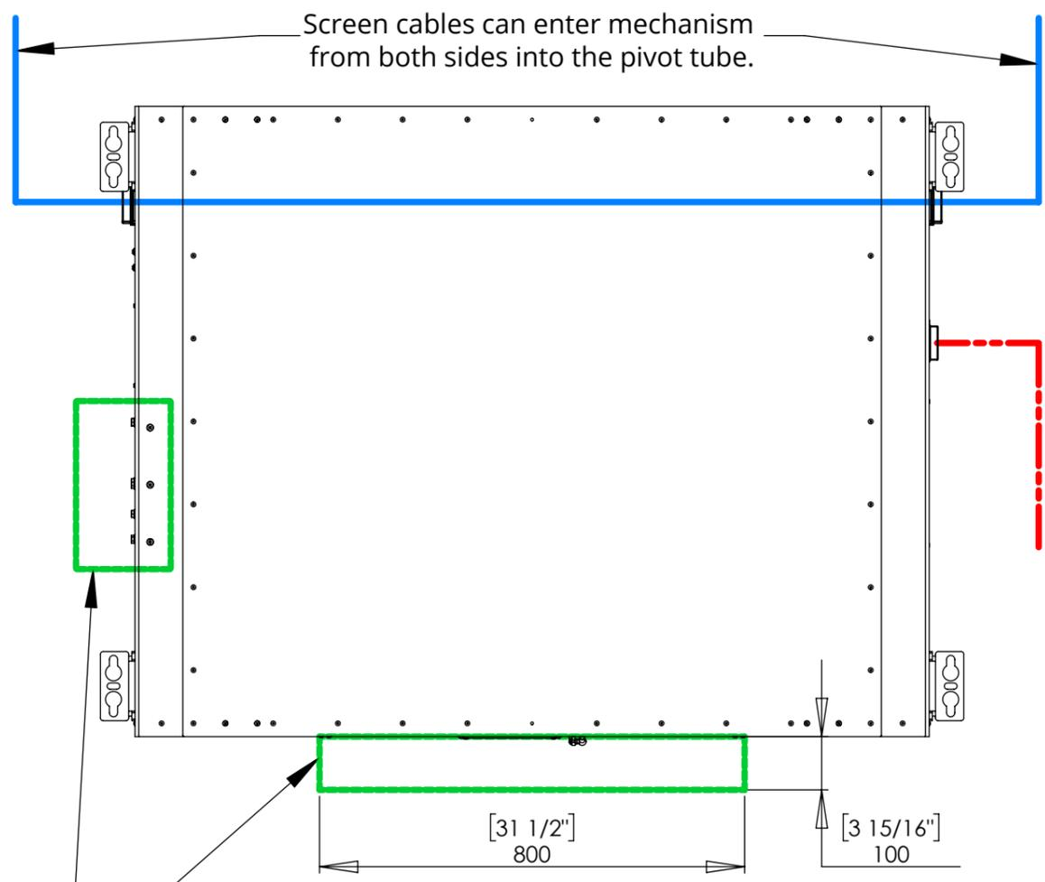
Screen cables can enter mechanism from both sides into the pivot tube.
