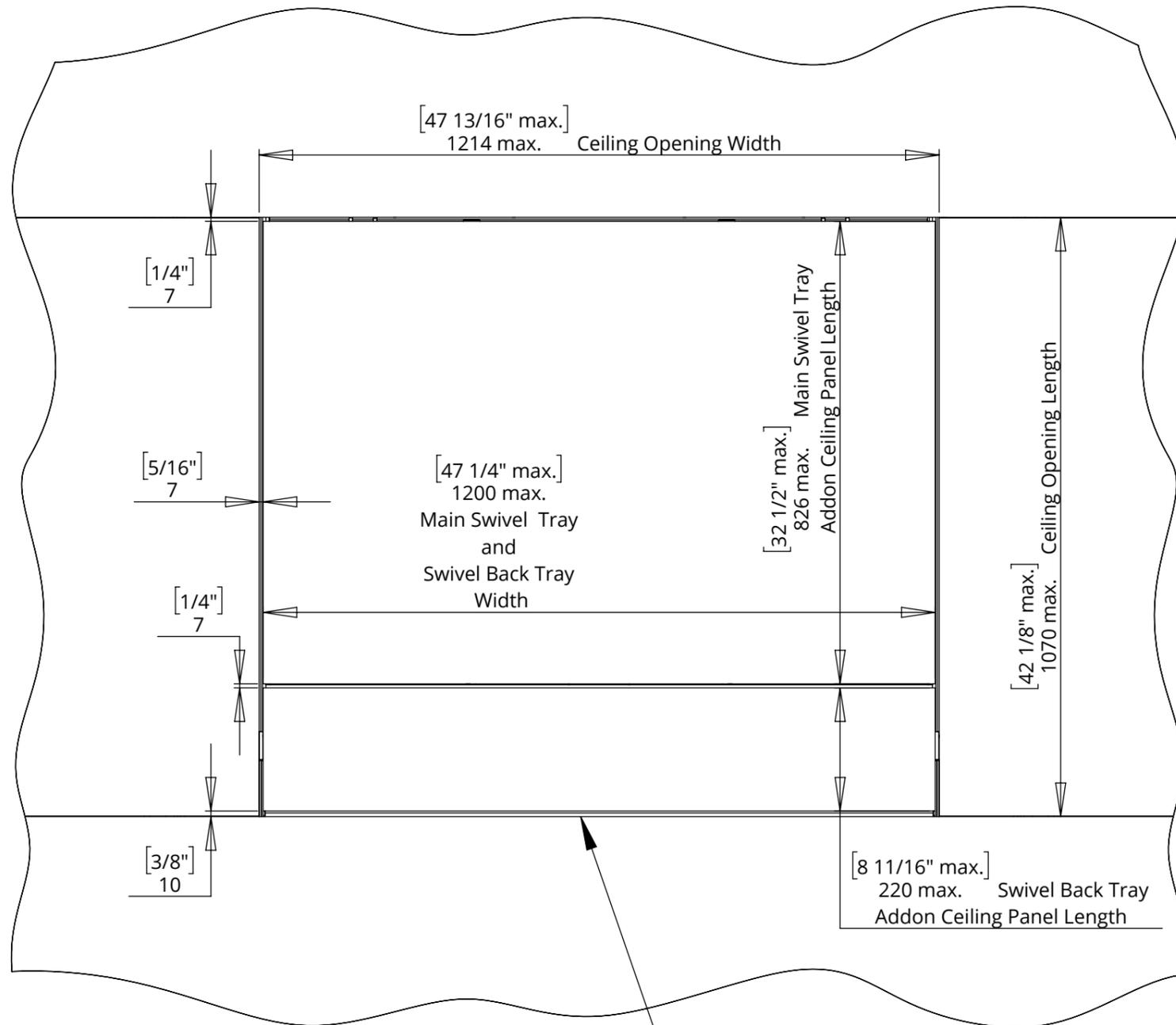
Mechanism designed to work with min. 7mm [0.3"] shadow gaps at front, sides & between addon panels
