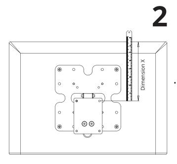
Measure from the top of the screen, down to the top mounting hole on the Wall Plate (Dimension X) to determine positioning of the top wall fixing holes.
