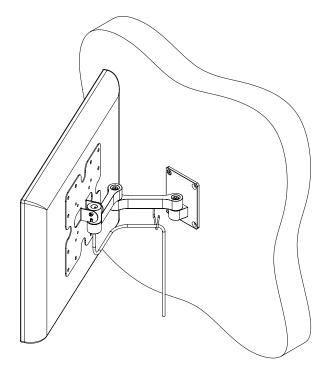
Run cables to the back of the TV and secure in place using the provide cable management hook.
