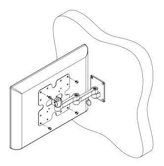
Fully extend the bracket and turn the FSA1 screen mount to 90° for better access. Hold the screen up to the FSA1 screen mount and fix in place using suitable fixings from the provided fixings pack.
