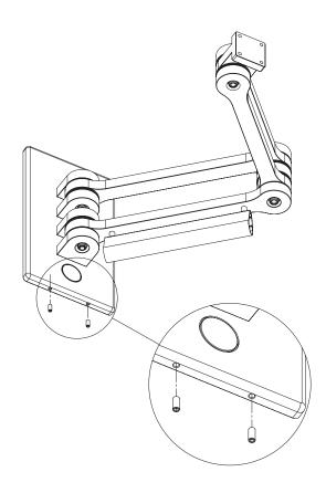
• Remove the 2 grub screws from the underside of the Wall Mount Plate.
