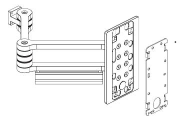
Separate the Wall Hook Plate from the Wall Mount by unhooking it.
