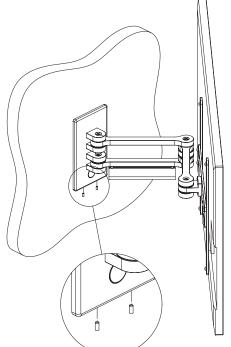
Secure the FSA3 bracket to the Hook Wall Plate by replacing the 2 grub screws in the bottom of the Wall Plate.
