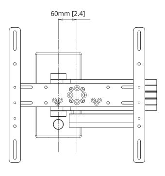
The center of the Wall Plate and the center of the Screen Plate are offset by 60mm, make sure you take this offset into consideration when mounting the FSA3 bracket.
