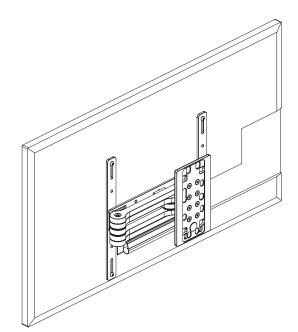
For screens with uneven backs or recess mount holes, the spacers in the fixings pack may be required.
