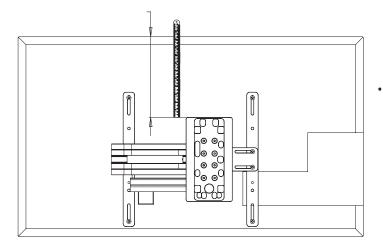
Measure the distance from the top of the screen to the top fixing holes in the Wall Hook plate to determine the correct height for the wall fixings.
