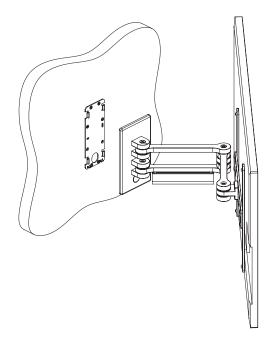
Once the Hook Wall Plate is secure, lift the FSA3 bracket and screen up onto the Wall Hook Plate.
