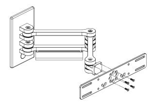
• Attach the Mount Cross Plate to the FSA3 Arms using the fixings provided as shown.
