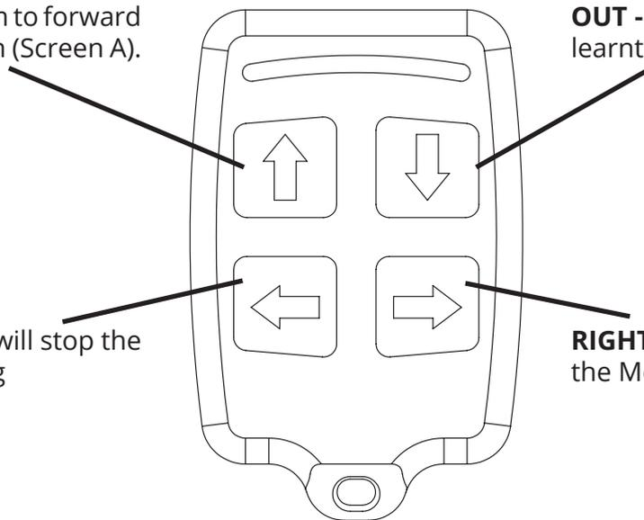
The Radio Frequency (RF) Remote Control can only be used to recall the above functions.
