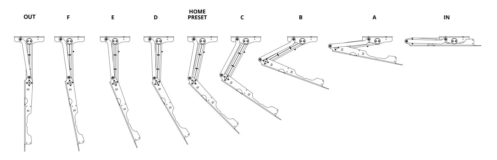
A number of preset positions are set in the mechanism which are shown above with the corresponding letter on the remote control.
