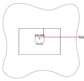
Separate the V2 Screen Plate and V2 Wall Plate and mark the desired wall mounting position using the distance measured in step 1.
