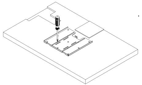
Place the V2 Screen Plate on to the back of the screen and fix in place using the bolts provided in the 'VESA Bolt / Spacer Pack'
