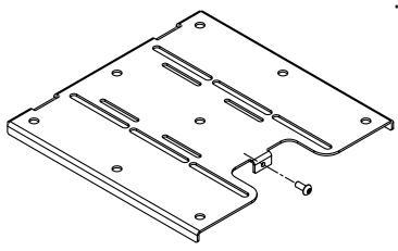
Remove the M5 Fixing Bolt and separate the V2 Screen Plate and V2 Wall Plate
