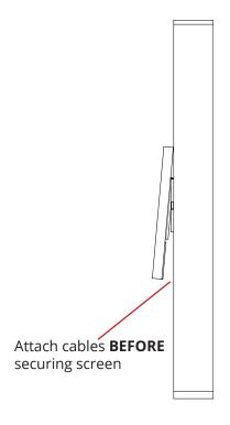
Hook the screen and V2 Screen Plate onto the V2 Wall Plate
