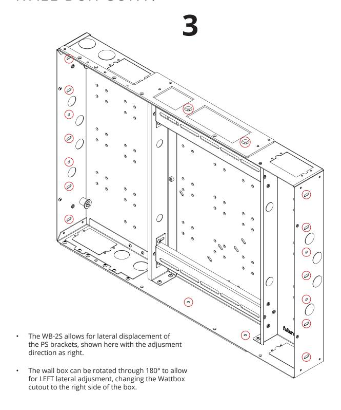
• The WB-2S should be inserted into the wall cut out from the front, then secured to the surrounding studs using the 40mm pozi head wood screws provided through the Ø6.5mm [0.25"] fixing holes circled below.
