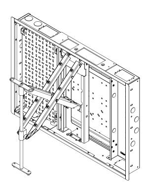
The larger shift side can be to the left or right depending on wall box orientation. Rotate the wall box 180° to determine shift direction.
